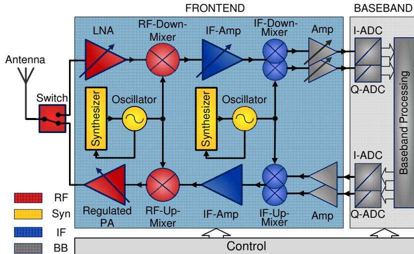
Fig. 1.5: System overview of a standard transceiver architecture.
