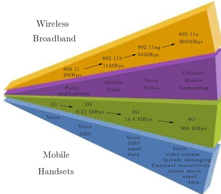
Fig. 1.1: Evolution of wireless communication standards.
