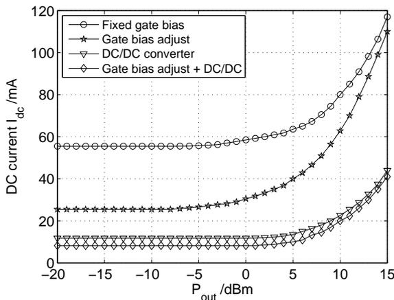
Fig. 1.9: Impact of PA regulation on  $I_{dc}$ .
