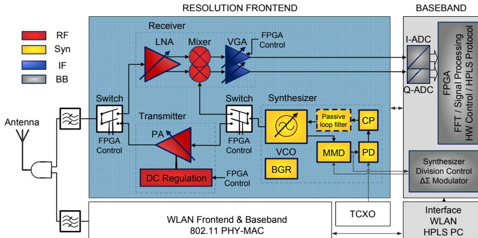
Fig. 1.6: System overview of the RESOLUTION transceiver architecture.
