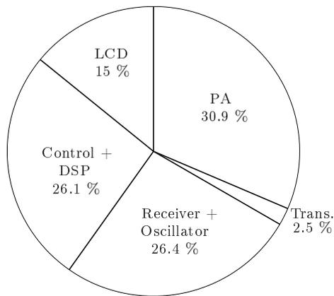
Fig. 1.7: GSM mobile terminal power budget, Trans. = Transmitter excluding PA.
